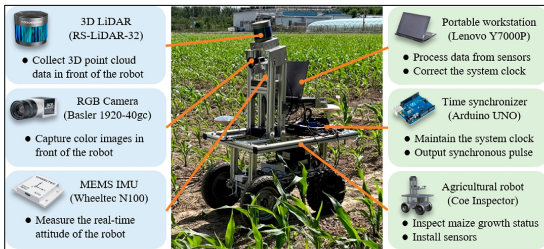
Figure 2. Multiple sensor device developed by Ban et al. Adapted from [30], © 2024, licensed under CC BY-NC-ND.
